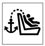
To assist you in locating the top tether anchors, the top tether anchor symbol is located near the top tether anchors.
